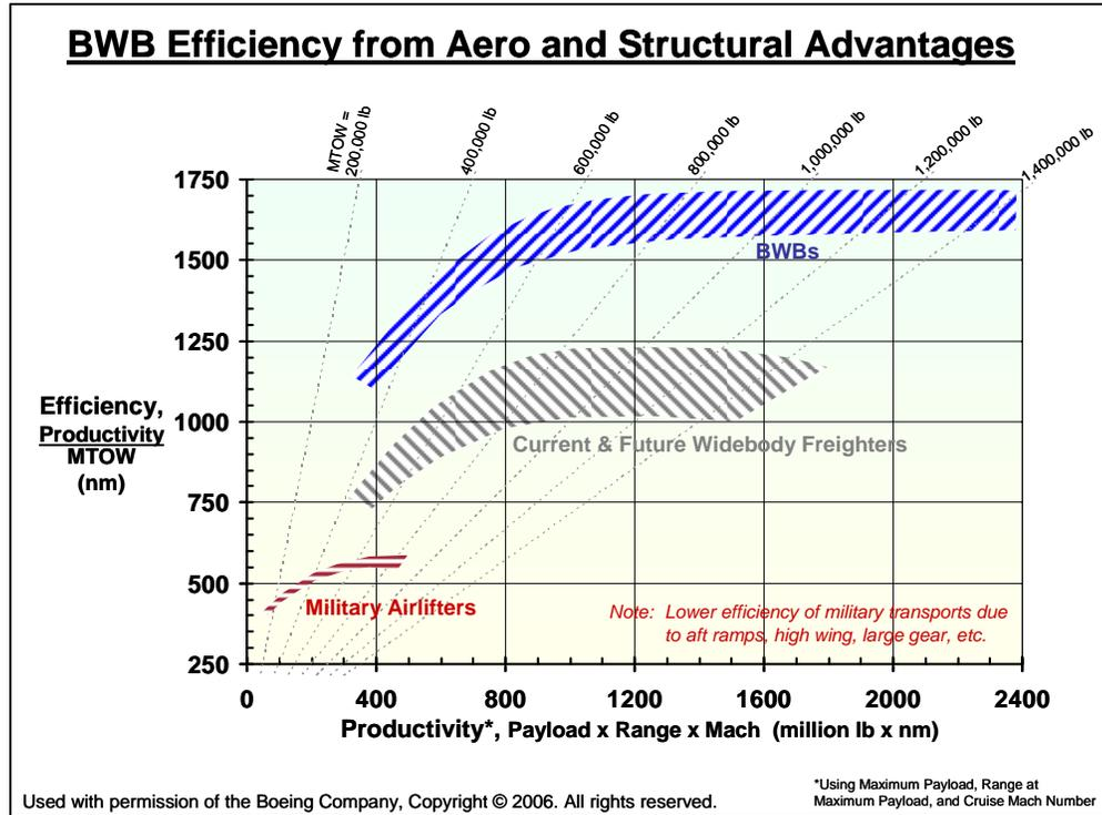
Figure 4.2: BWB Efficiency from Aero and Structural Advantages
