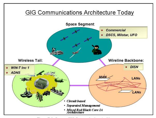
**Figure E-2: Current GIG Communications Architecture**
