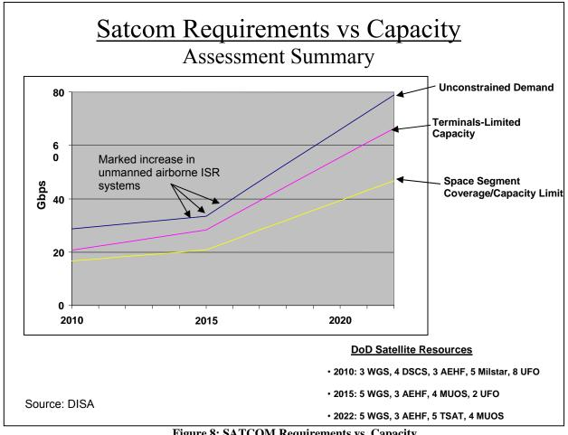
Figure 8: SATCOM Requirements vs. Capacity
