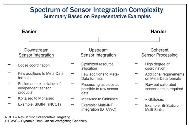
**Figure 5: Spectrum of Sensor Integration Complexity**
