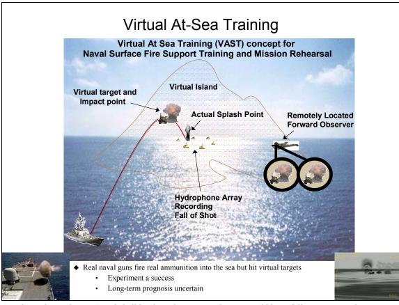
A real naval gun shoots. A real shell lands in the ocean. Where it would have fallen on a virtual target is calculated and inserted into the view of a real forward gunfire observer. The parts that require training are real; much of the rest is simulated but can be exercised separately. We could wish that future funding were as real as the gunfire and the communication networks.
