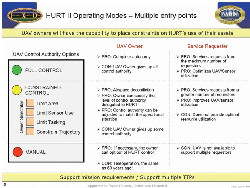
In addition, HURT developed data formats to determine the minimum communication requirements for sharing tasking and defined constraints around the network to allow integration of coordinated tasking systems. HURT operating modes show operator ability to dial in full manual control of assets to full autonomous control, with intermediate levels of constrained control possible. Pros and cons of each level are shown in Figure 11.
