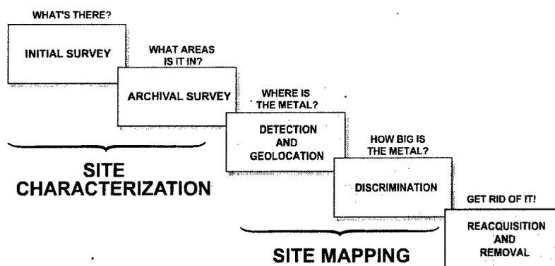
Figure D-1. Elements of the UXO Cleanup Process
