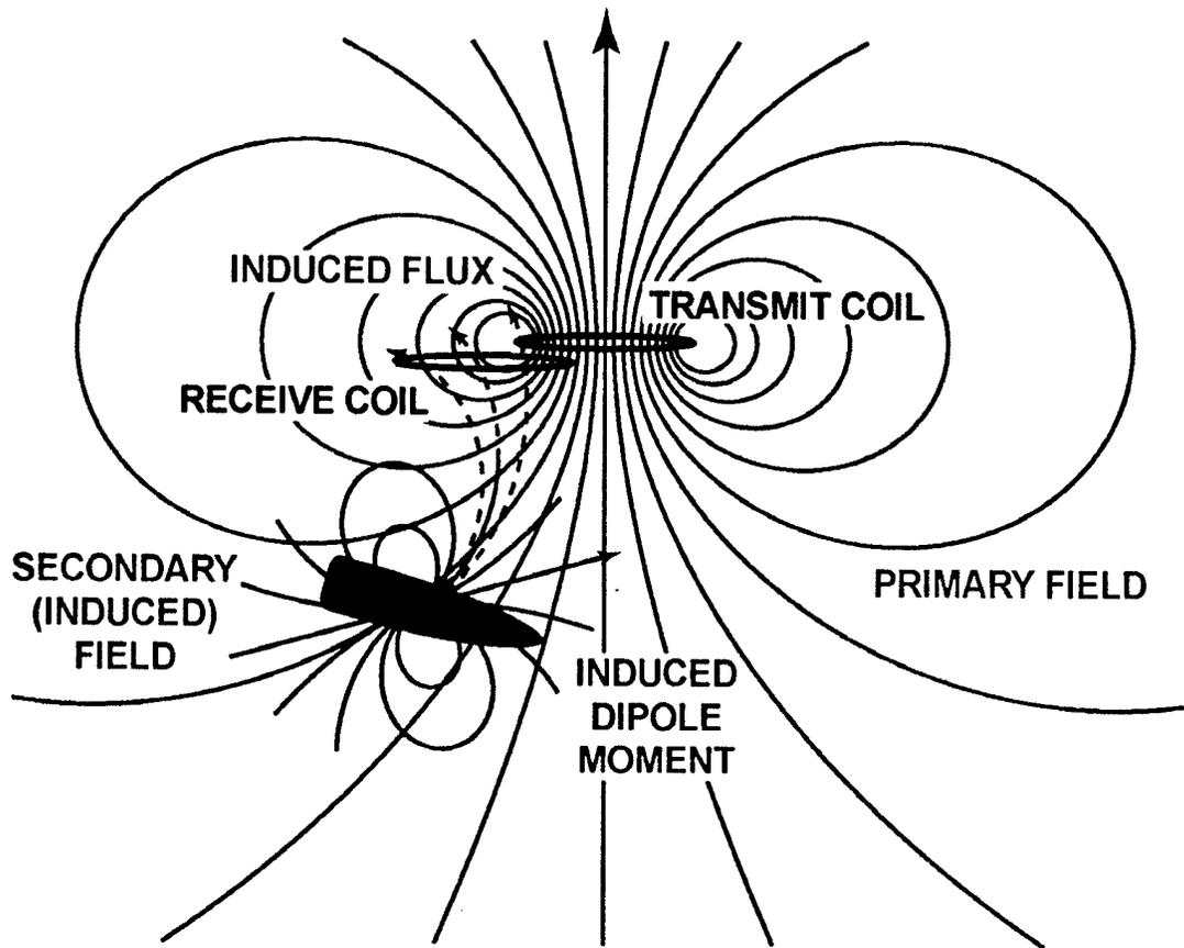
Figure D-10. Electromagnetic Induction (EMI)
